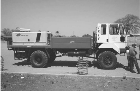
Auxiliary truck for pumping water down through the drill bit
